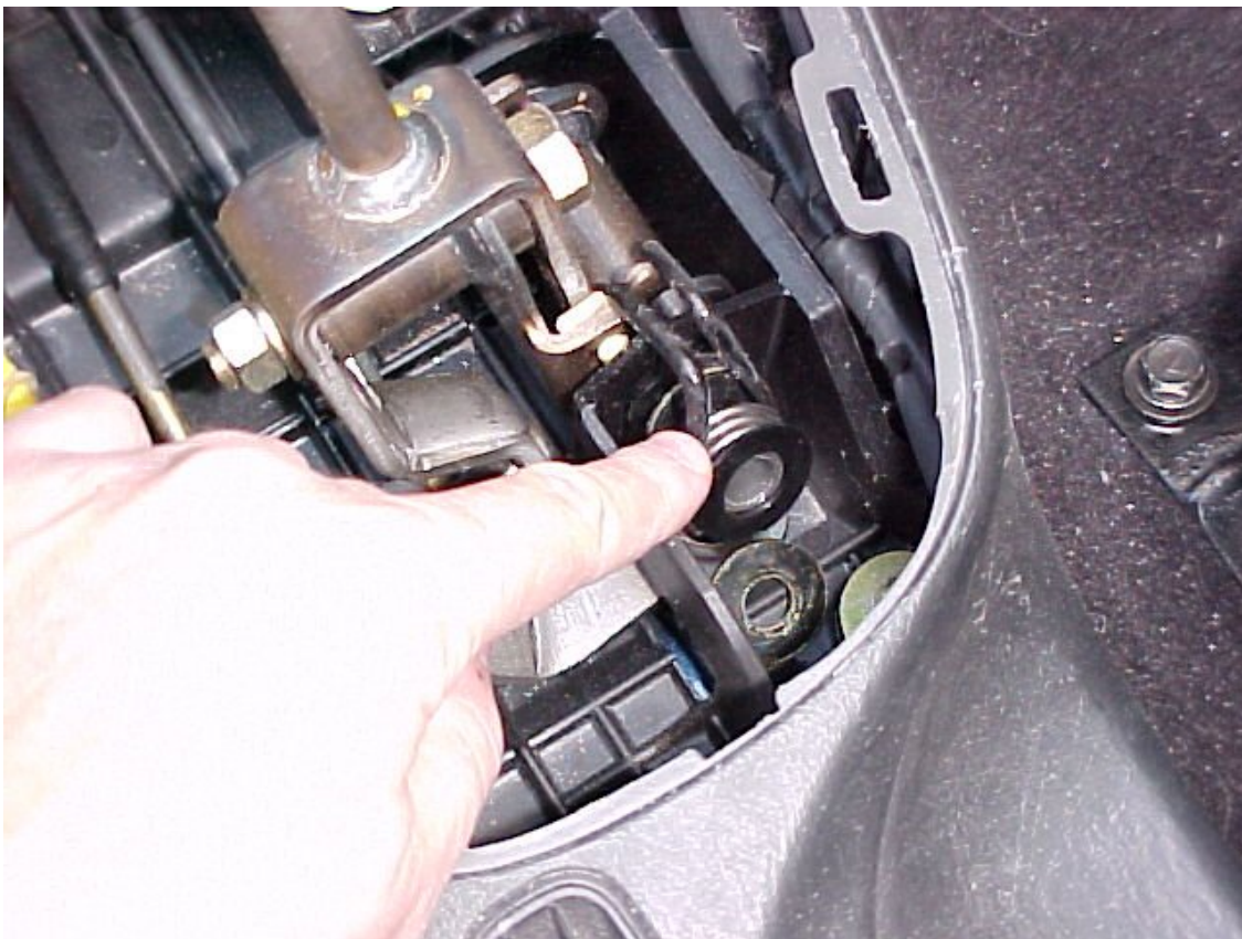
9) Remove the shifter return spring and bushings.
