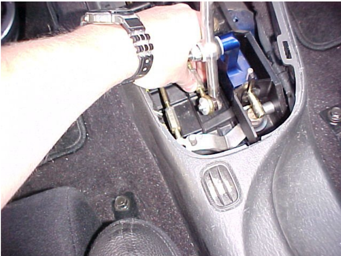
15) Install the shift cable onto the pin at the bottom of the shift lever.
