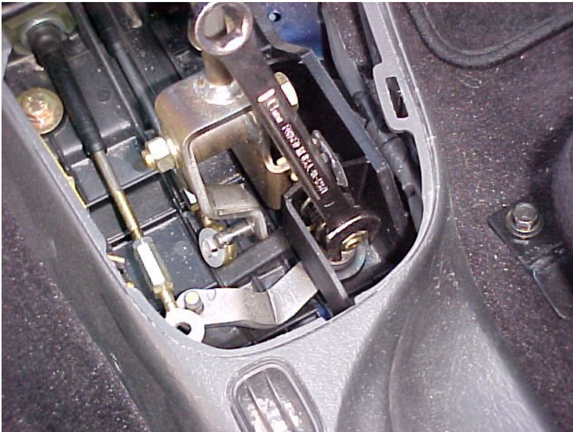
7) Remove the nut from the shift shaft with an open-ended wrench.
