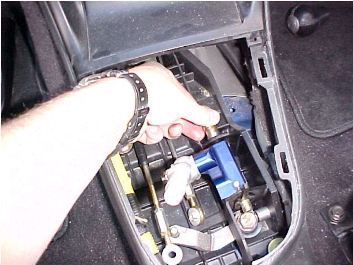
14) Re-insert the shift shaft from the front of the shifter assembly.
