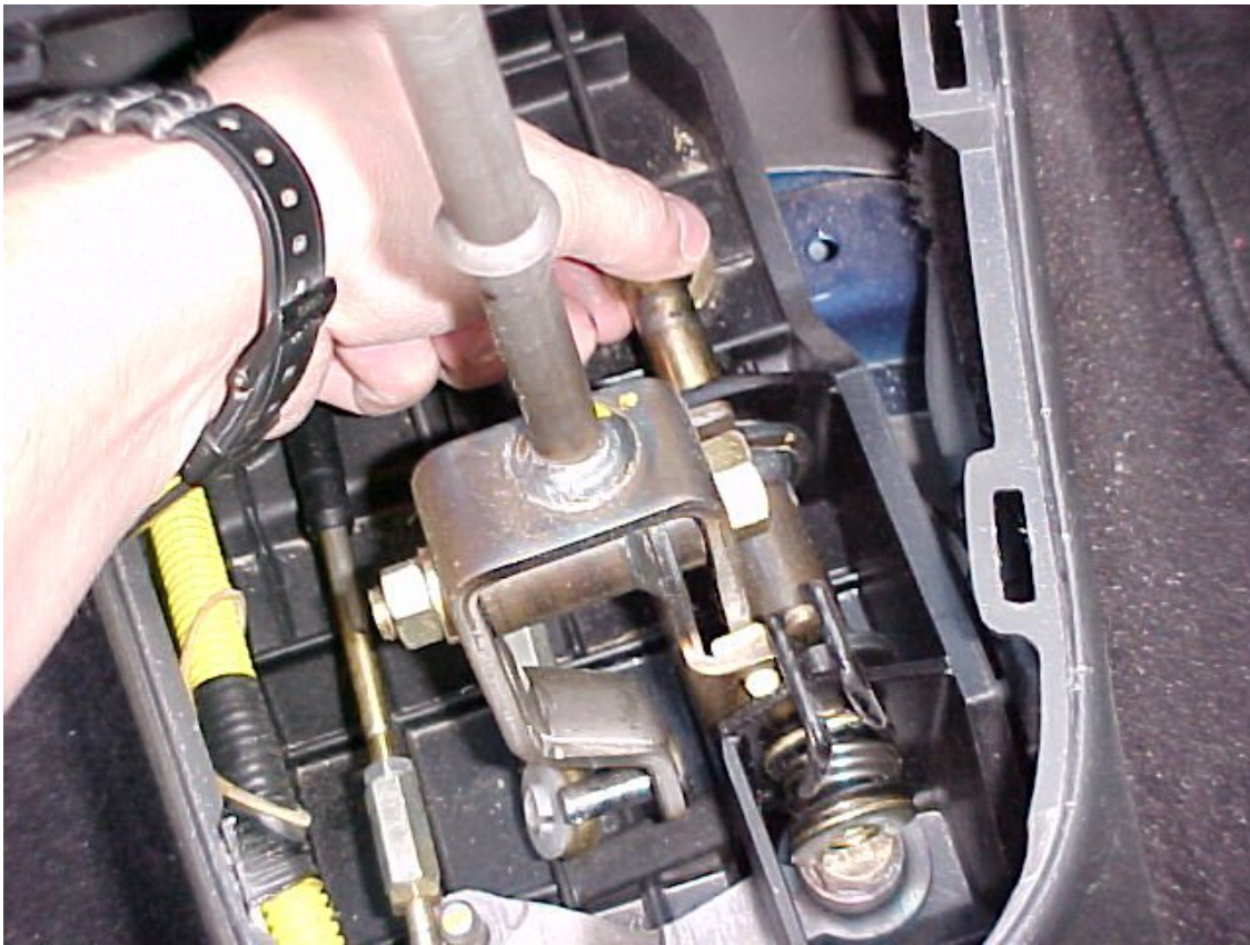
8) Pull the shift shaft out the front of the shifter assembly.
